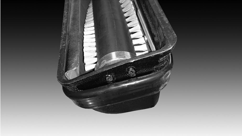
3. With a 10mm wrench, secure the nut inside of the brush roll and use a 4mm Allen wrench for the screw. Loosen screws to release the brush from the vacuum.
